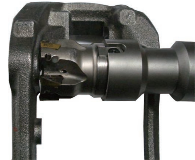
Application: Side milling Solution: Achteck AP series
