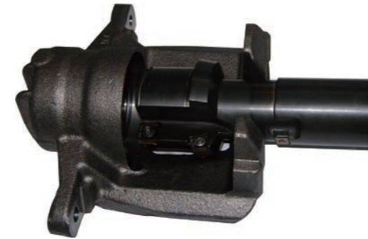
Application: Piston hole rough boring Solution: Achteck special cutter+standard insert
