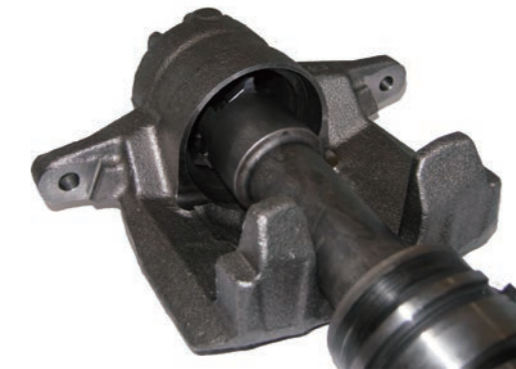
Application: Groove milling internal grooving piston hole Solution: Achteck insert + special cutter
