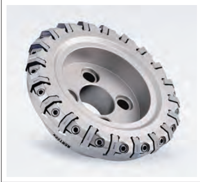
AFM45-XN09-W milling cutter with heptagon inserts, extra close pitch with wedge clamping, combined with heat resistant CVD coated inserts. The ideal choice of cast iron rough milling.
