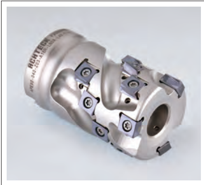
APE90-LN09/LN13 porcupine milling cutter uses tangential insert with helical edge profile. The high strength insert have 4 cutting edges, offering high productivity, machining reliability and cost efficiency.
